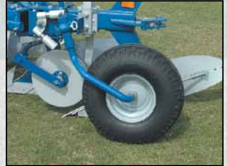
Roue combiné transport/jauge 10.00x12, diam. 710mm, largeur 264mm.
